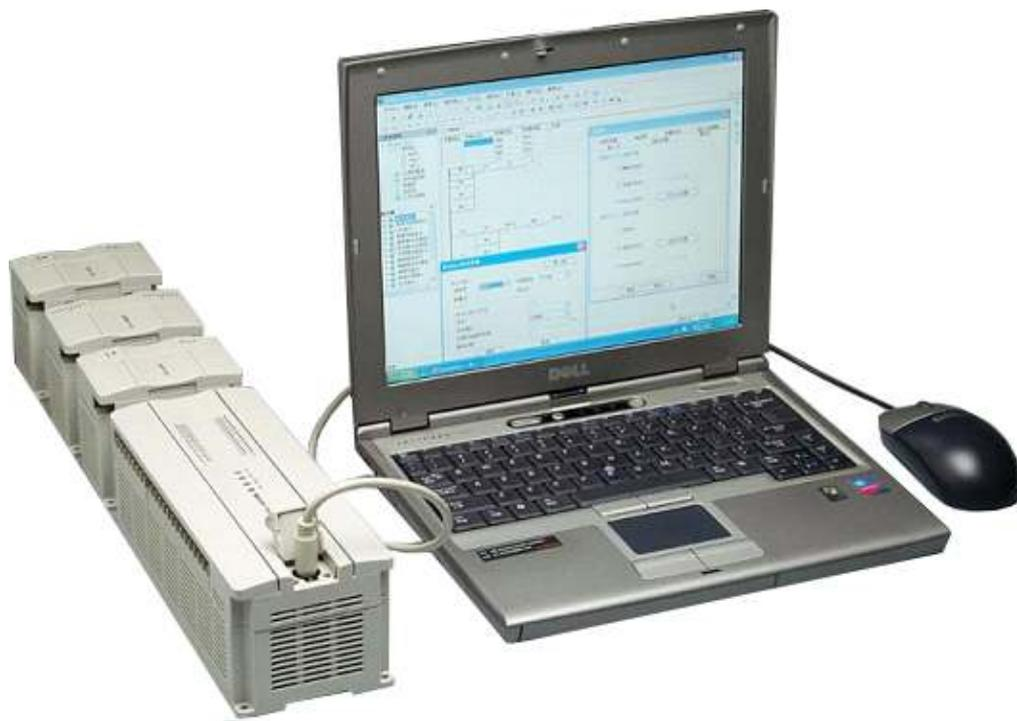
Figure 1-4 Connection of programming cable
