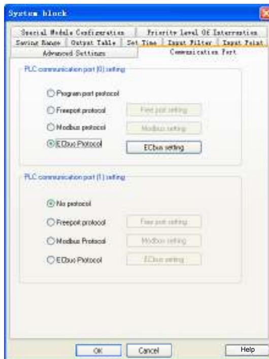
Figure 2-4 Setting communication ports
