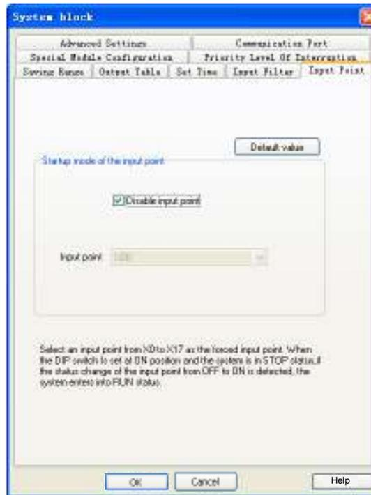
Figure 2-8 Setting input point
