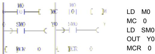
When M0 = ON, the instructions in the MC 0 - MCR 0 structure will be executed, and Y0 = ON. When M0 = OFF, the instructions in the MC 0 - MCR 0 structure will not be executed, and the bit element Y0 designated by the designation operand of the OUT instruction in the structure will be cleared, Y0 = OFF.
